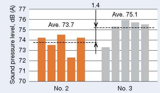
Fig. 29 Sound pressure levels measured by vehicle running tests with the EPS No. 2 and No. 3. Five measurements were done with each EPS.
