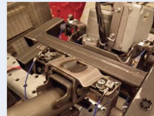
(c) 3-axis accelerometers on the connections of steering column (No. 3, 4, 5, 6)
