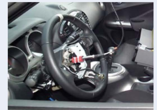
Fig. 3 Microphone mounted at the steering wheel center from which the airbag module has been removed
