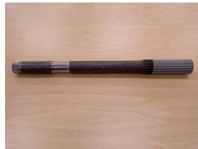
Photo 2 New hollow structure shaft
