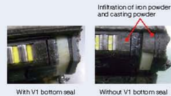
Photo. 5 Infiltration of foreign particles
