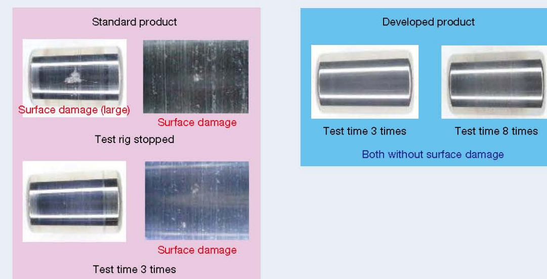
Fig. 7 Bearing endurance test results
